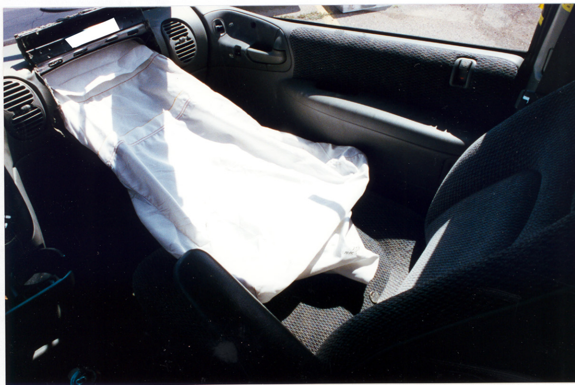
82. View of the rearward extension of the passenger side air bag.
